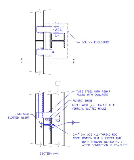
NOTE: THE ENGINEER OF RECORD SHALL CHECK THE COLUMN FOR LOCALIZED BUCKLING
