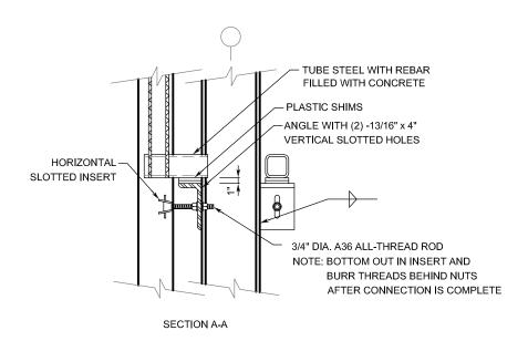
NOTE: THE ENGINEER OF RECORD SHALL CHECK THE COLUMN FOR LOCALIZED BUCKLING
