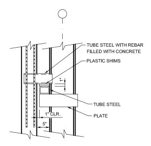
NOTE: THE ENGINEER OF RECORD SHALL CHECK THE COLUMN FOR LOCALIZED BUCKLING
