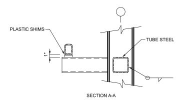
NOTE: THE ENGINEER OF RECORD SHALL CHECK THE COLUMN FOR LOCALIZED BUCKLING
