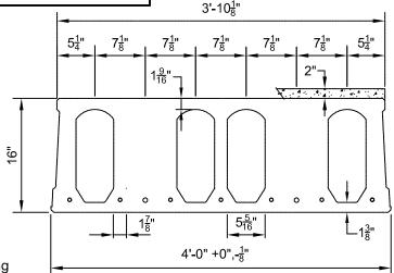
Allowable Live Load = (1.6)(Load Table Value) - (1.2)(Superimposed Dead Load)
