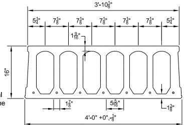
Allowable Live Load = (1.6)(Load Table Value) - (1.2)(Superimposed Dead Load)
