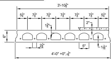
Allowable Live Load = (1.6)(Load Table Value) - (1.2)(Superimposed Dead Load)
