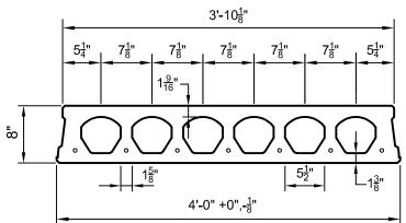
Allowable Live Load = (1.6)(Load Table Value) - (1.2)(Superimposed Dead Load)
