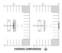
As mentioned earlier in this narrative, in parking structures associated with adjacent "wrap structures" it is common for the precast fire barrier wall panels to also serve as shear walls. This is graphically shown below.
